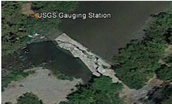
This failing cement apron is part of a gauging station used to measure stream flow in Alameda Creek. It is impassable to steelhead trout and other native fish at low flows. A new gauging station is in place, but continued use of this gauge allows scientists to properly calibrate the new data with historic.
