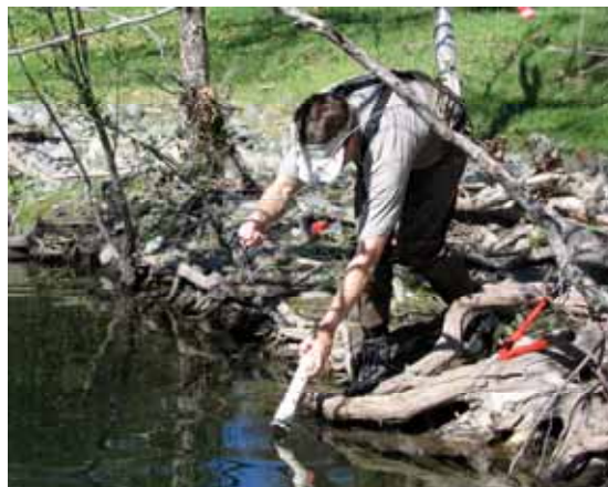
Figure 5-2. Scott Chenue, NRLMD Biologist III, deploying temperature sensor in Alameda Creek.
