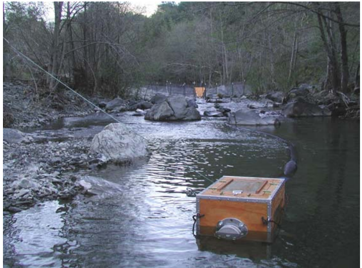
Figure 7. Arroyo Hondo trapping site – trap for downstream migrating fish, looking in an upstream direction.
