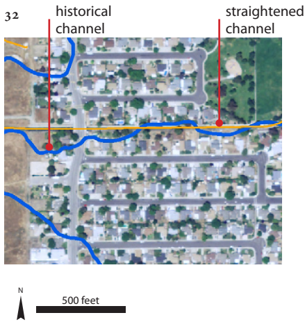
Figure 2.3. Change in sinuosity. The historical course of Arroyo las Positas, shown in blue, was much more sinuous than the present-day course, shown in orange. However, as the two lines fall within 50 feet over much of their length, these segments would be recorded as no change in our analysis of positional change, although we did capture the historical course in our historical stream network. (USDA 2009)
