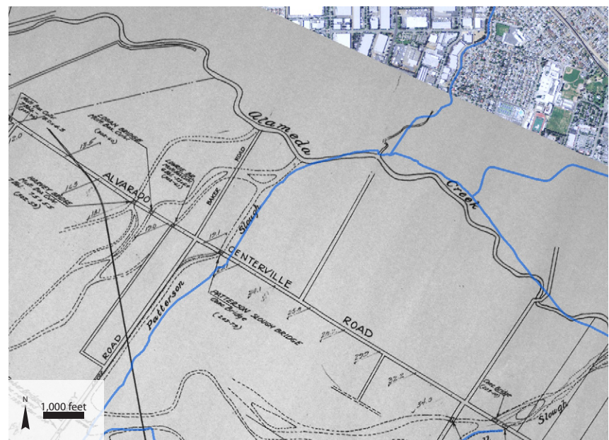
Figure 6.51. The Splits and the Alameda Creek Flood Control Channel. This 1915 map shows the newly created Splits channel (labeled Patterson Slough), which lines up with the present-day Flood Control Channel, shown in blue. The multi-thread pattern of the Splits channel reflects the semi-natural processes that created it. See also figure 6.48. (Unknown 1942, courtesy ACWD)
